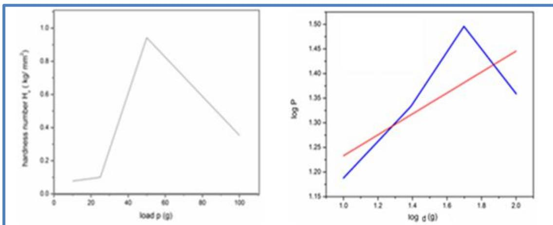
Fig.5a. Variation of HV vs. Load of PHF crystal
