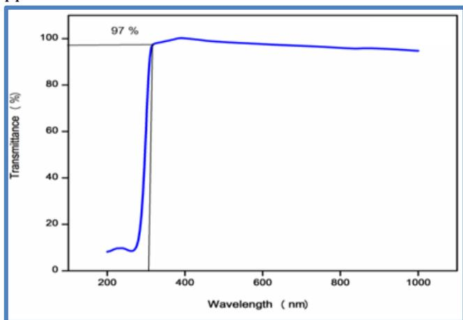
Fig.2. UV-Vis transmittance spectrum of PHF crystal
