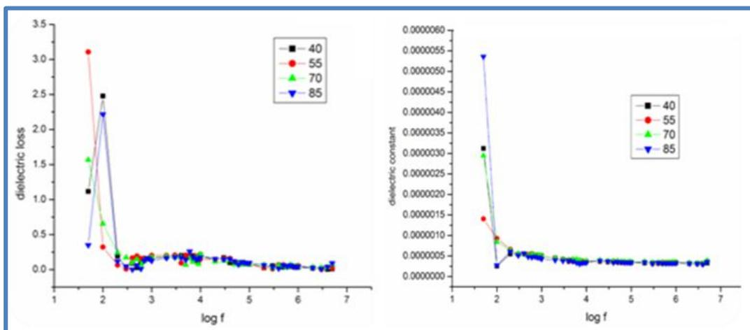
Fig.4a. Log f vs. dielectric loss of PHF
