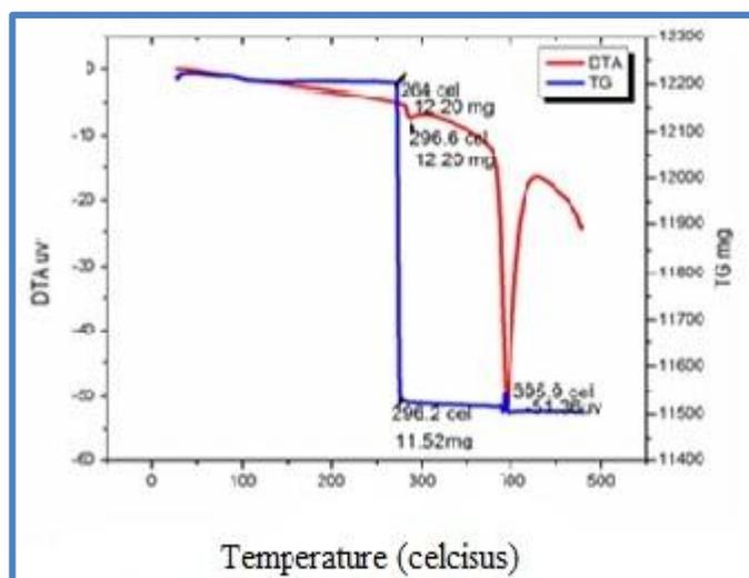
Fig. 3 Thermal Analysis (TG-DTA) PHF Crystal
