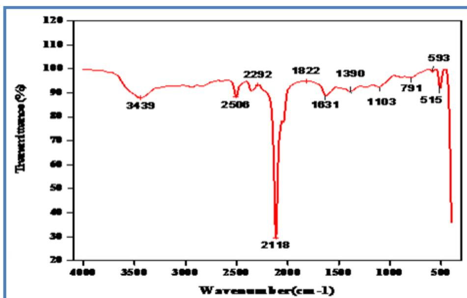
**Fig.2.** FT-IR Spectrum of pure PHF crystal
